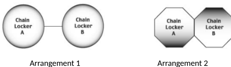
Figure 18.3: Chain locker arrangement
