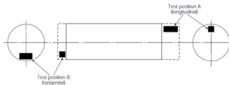
Figure 6.1: Location of specimens in unflanged shafts and rods
