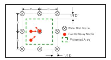
For this system, the outer nozzles should be installed outside of the protected area a distance of at least 1/4 of the maximum nozzle spacing.
