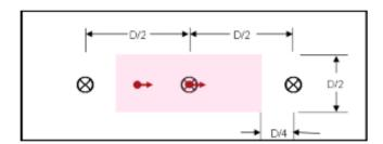
For this system, the outer nozzles should be placed outside of the protected area a distance of at least 1/4 of the maximum nozzle spacing.
