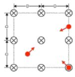
For this system, outer nozzles can be located either at the edge of the protected area or outside of the protected area.
